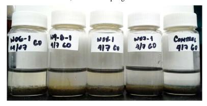
**Figure 1. Gel-stabilized gradient tube cultures.** Gel-stabilized gradient tubes inoculated with samples from biofouled wells. Tubes with IOB-containing samples (W9-B-1; W07-1; W08-1 – described in Table 1) develop a faint orange ring of biogenically produced ferric oxides within the clear (oxic) phase, right above the dark (anoxic, rich in Fe<sup>2+</sup>) phase. Tubes inoculated with non-IOB samples (W06-01 – described in Table 1) remain unchanged as does the un-inoculated control.
